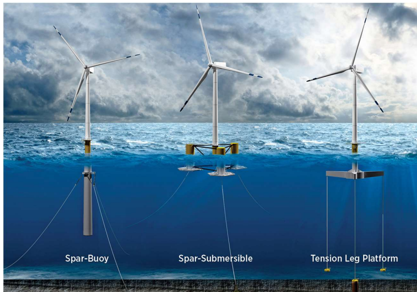
Joonis 1: Meretuulike ujuvundamenditüübid. Allikas: Illustration by Joshua Bauer, National Renewable Energy Laboratory (US Department of Energy)
