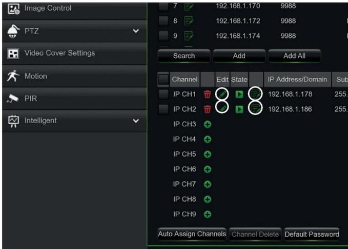
To change the network parameters of the connected camera (e.g.: camera IP address from DHCP to static, mask, Gateway, port) select the button (circled in red in the previous image).
