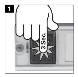
Press the wireless bell button and keep it pressed for 3 seconds. The **red** indicator **flashes** at the wireless bell button.
