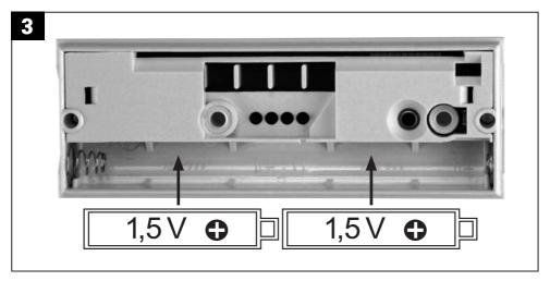
Insert 2 x 1.5 V (AAA type) batteries into the bottom part of the wireless bell button. Note the polarity (see markings).
