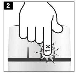
Then, press the **Menu button** on the wireless chime in its normal state once.
