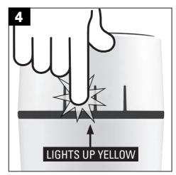
Press the **Select button** to end the slumber function prematurely. As confirmation, the LED ring **lights up yellow** while you press the button.
