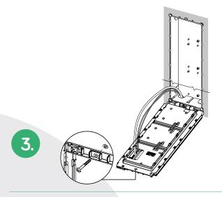
Connect the two wires of the 2Voice riser and those of the electric lock, fixing all with the other screw on the wall frame upper side.
