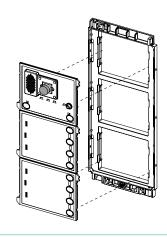
Then insert the various snap-fit modules on the wall frame and connect them together using the supplied flat cables.
