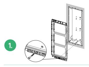
Using the screw supplied with the product, fix the lower part and the module holder wall frame, on the flush-mounting box on the wall.
