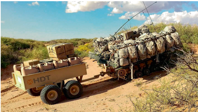
Picture 2: A combat loaded SMET concept transport vehicle. Two of these systems were used to haul an infantry platoon’s equipment during field-testing 16
