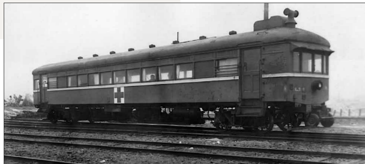
One of the self-propelled "doodlebugs" operated by the U.S. Army Medical Corps in Korea. Built in Japan, the gasoline-powered cars were based on American designs of the 1920s and 1930s. U.S. Army Transportation Museum Collection, Fort Eustis, Virginia
