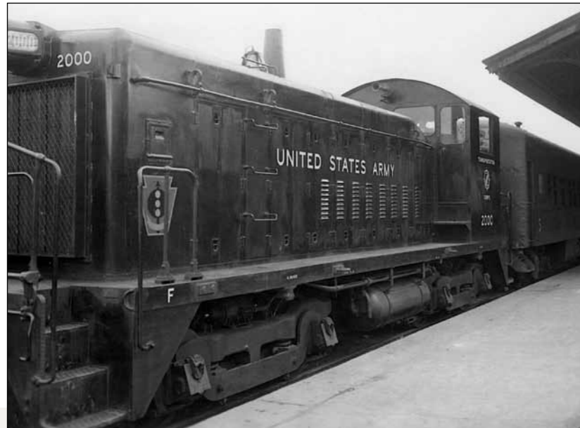
SW8 No. 2000 departs Pusan, Korea, for Seoul with the EUSAK Express on July 9, 1951. This was the first run of a diesel-electric-powered passenger train on the Korean peninsula. The keystone insignia represents the 724th Transportation Railway Operating Battalion, which was a Pennsylvania Railroad-sponsored reserve unit activated in August 1950 for service in Korea. The 712th Transportation Railway Operating Battalion (a Reading Railroad-sponsored reserve unit) was also activated in August 1950 for Korean service. Both battalions drilled in Philadelphia before being activated. U.S. Army Signal Corps Collection, U.S. National Archives
