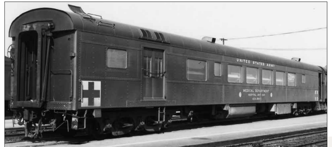
A U.S. Army hospital car built by American Car & Foundry in 1944. These cars' 84-foot length and six-wheel trucks combined to limit their usefulness during the Korean War. Robert J. Wayner Collection
