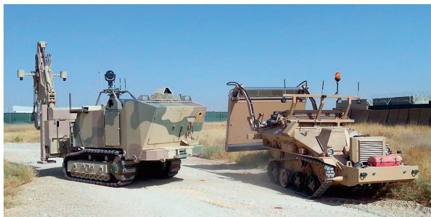
Picture 1. UGVs used in Route Clearance System in Afghanistan.
