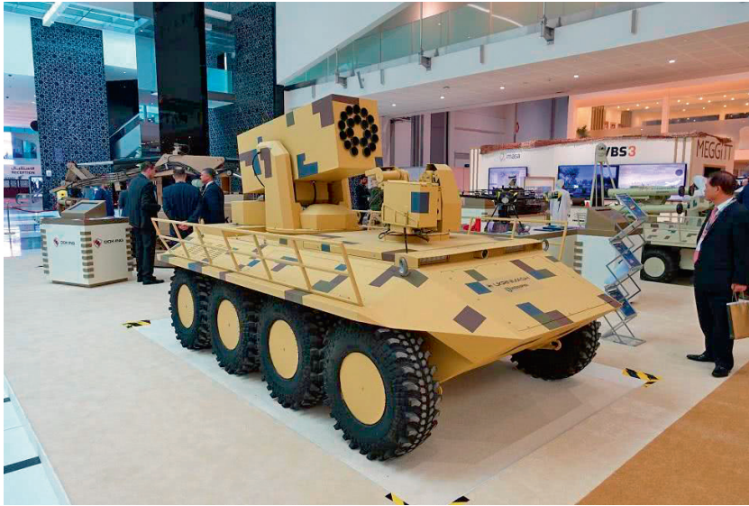
Picture 3. 8×8 Phantom-2 unmanned ground vehicle.
