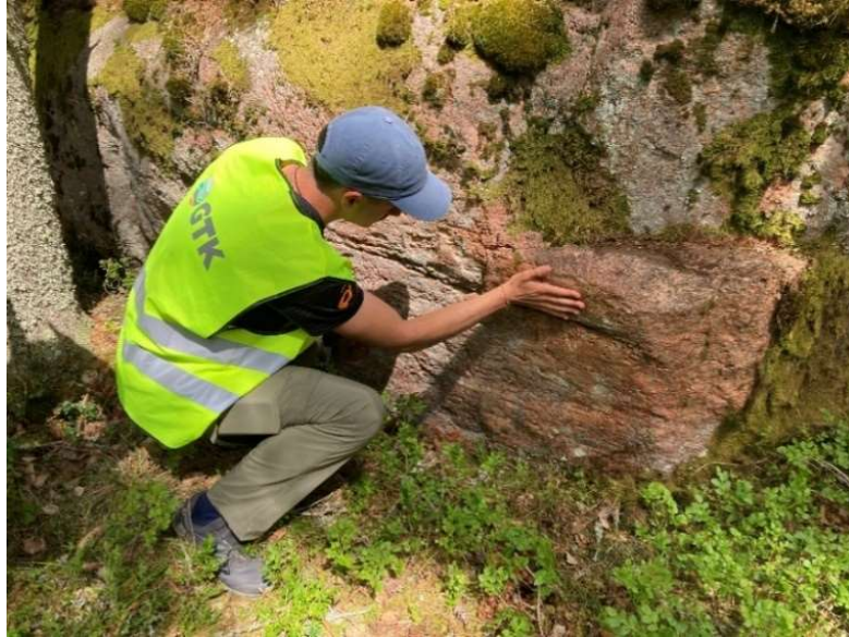
Figure 4. An outcrop-overview of a right-lateral strike-slip fault associated with zeolite, prehnite and chlorite alteration.
