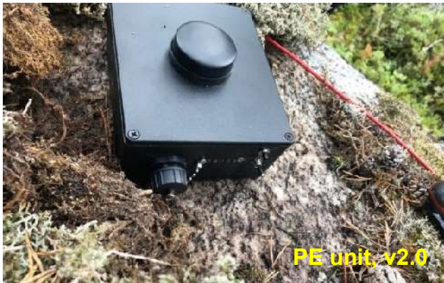
Piezoelectric seismograph Geological Survey of Norway
