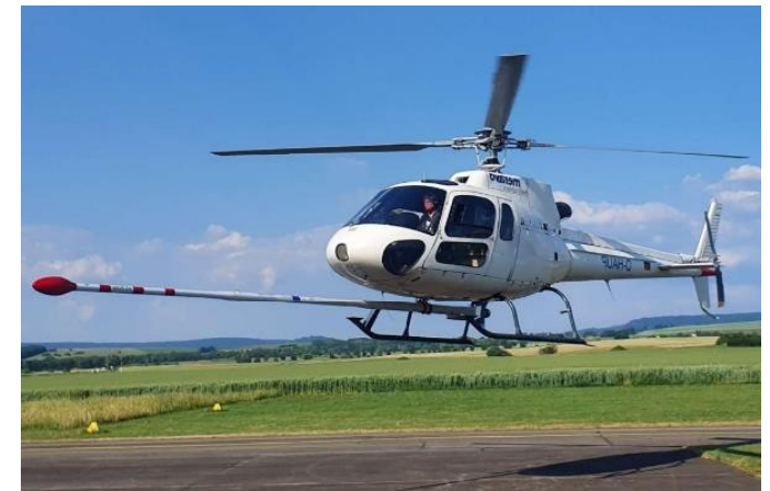
EASA-certified, helicopter-compatible nose stinger magnetometer/radiometer terratec Geophysical Services GmbH
