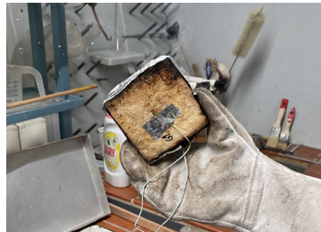
Mycelium material can withstand heat and flame
