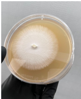
Mycelium acts as a glue and binds different leftovers into strong solid materials
