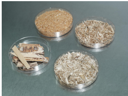
Mycelium acts as a glue and binds different leftovers into strong solid materials
