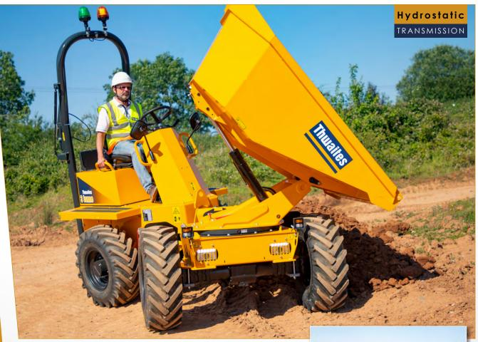
The Thwaites 3 Tonne Power Swivel, Stage V dumper is manufactured with contractors and hirers in mind - ensuring operator safety, reducing risk on site and improving performance. Powered by an 18.4 kW 3-cylinder Yanmar engine, delivering 107 Nm max torque for optimum traction and control, this machine is driven by a Hydrostatic transmission, making it simple and straightforward to operate.
