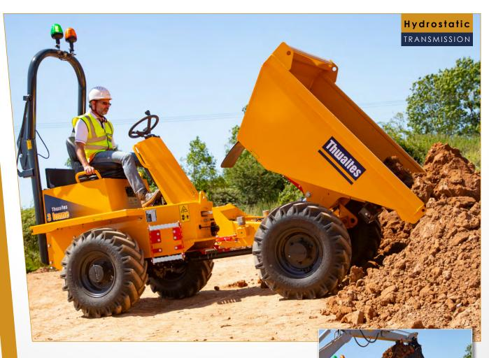
The Thwaites 3 Tonne Front Tip, Stage V dumper is manufactured with contractors and hirers in mind – ensuring operator safety, reducing risk on site and improving performance. Powered by an 18.4 kW 3-cylinder Yanmar engine, delivering 107 Nm max torque for optimum traction and control, this machine is driven by a Hydrostatic transmission, making it simple and straightforward to operate.
