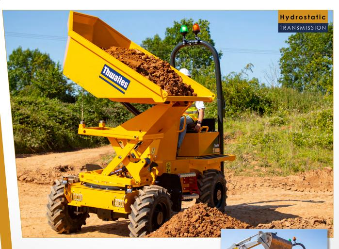
The Thwaites 2 Tonne Hi Swivel, Stage V dumper is manufactured with contractors and hirers in mind - ensuring operator safety, reducing risk on site and improving performance. Powered by an 18.4 kW 3-cylinder Yanmar engine, delivering 107 Nm max torque for optimum traction and control, this machine is driven by a Hydrostatic transmission, making it simple and straightforward to operate.
