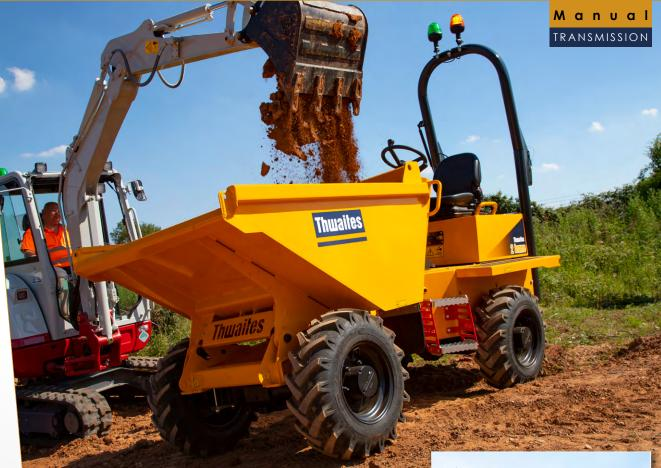
The Thwaites 2 Tonne Front Tip, Stage V dumper is manufactured with contractors and hirers in mind – ensuring operator safety, reducing risk on site and improving performance. Powered by an 18.4 kW 3-cylinder Yanmar engine, delivering 107 Nm max torque for optimum traction and control. This machine is driven by a Manual transmission.
