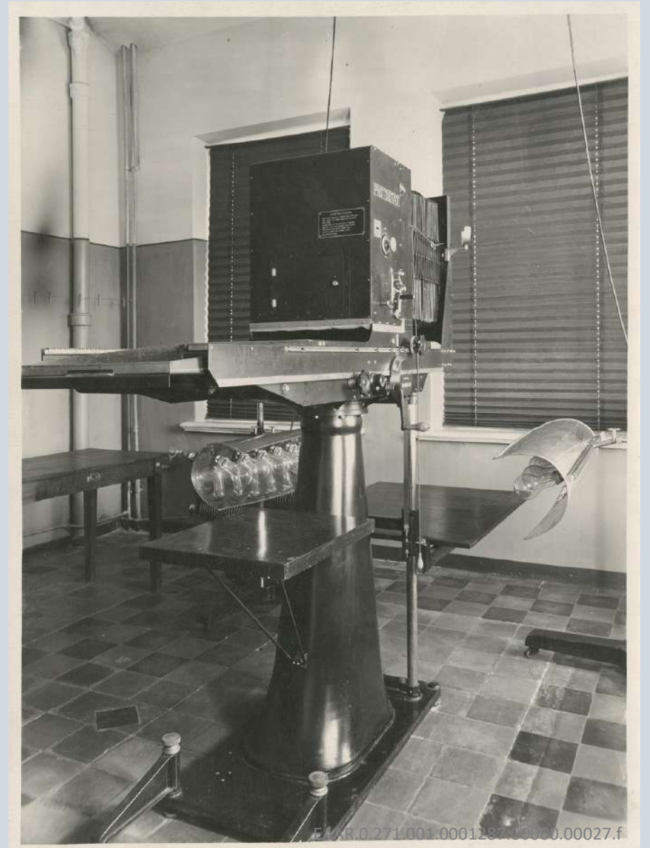
Figure 38 Photostat camera illustrated in Modern Plan Copying by B. J. Hall, London, 1935
