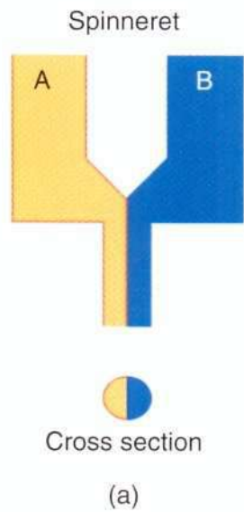
Figure 6.9 Bicomponent fiber structure: (a) bilateral, (b) core-sheath, (c) matrix-fibril.
