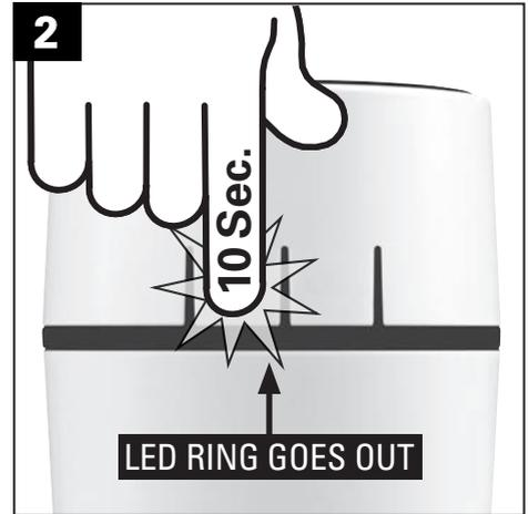
Press the **Select button** within **7 seconds** and keep it **pressed for 10 seconds**. The LED ring goes out as confirmation.
