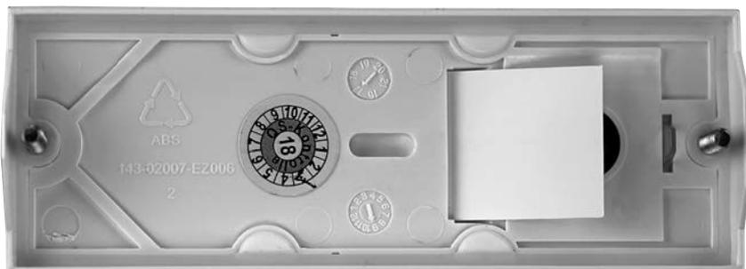
To label, pull the nameplate out at the side and then push it back in again. Use the hexagon socket screws to screw the top part of the wireless bell button firmly onto the bottom part.
