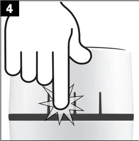
Now, press the **Select button** until the LED ring lights up in the required colour. Your selection **is saved automatically** if no button is pressed for **7 seconds**.
