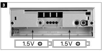
Insert 2 x 1.5 V (AAA type) batteries into the bottom part of the wireless bell button. Note the polarity (see markings).
