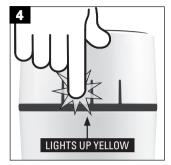
Press the **Select button** to end the slumber function prematurely. As confirmation, the LED ring **lights up yellow** while you press the button.
