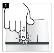
Press the **Select button 2, 3 or 4 times** at one second intervals in the normal state to activate the slumber function for **1, 3 or 9 hours**.
