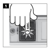
Press the wireless bell button and keep it pressed for 3 seconds.
