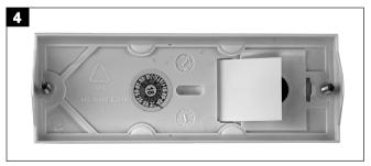
To label, pull the nameplate out at the side and then push it back in again. Use the hexagon socket screws to screw the top part of the wireless bell button firmly onto the bottom part.
