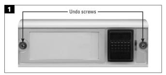
Use the Allen key to undo the screws in the cover of the wireless bell button, and then remove the top half.
