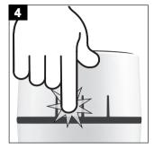
Now, press the **Select button** until the LED ring lights up in the required colour. Your selection **is saved automatically** if no button is pressed for **7 seconds**.
