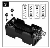
Insert  $4 \times 1.5 \text{ V}$  (AA type) batteries into the battery holder. Note the polarity.
