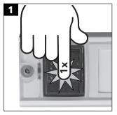
Press the wireless bell button to set the colour of the LED ring on the wireless chime.
