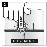
Press the Select button within 7 seconds and keep it pressed for 10 seconds. The LED ring goes out as confirmation
