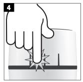
Press the **Select button** until the melody is played with the required volume. Your selection is saved **automatically** if no button is pressed for **7 seconds**.
