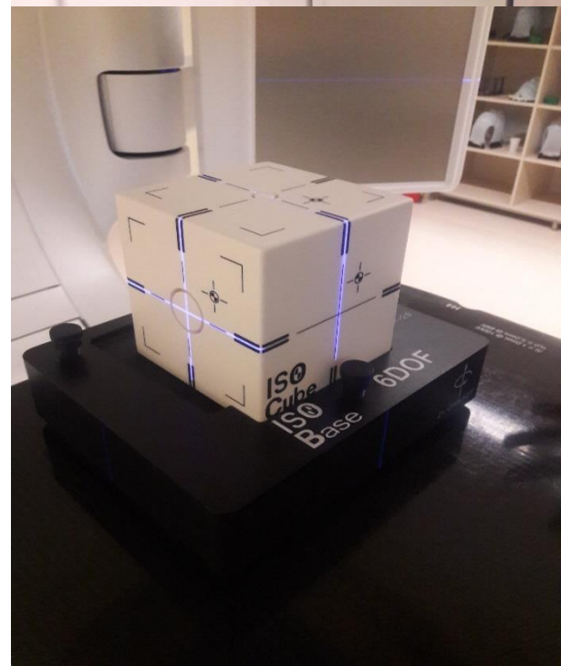
Tests on linac to ensure 1 mm accuracy
