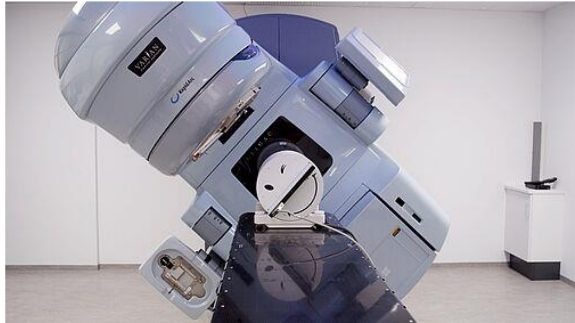
Treatment plan check with plate detector (>1000 mini ion chambers) under linac
