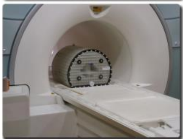
MRI testing – main aspect –geometric distortion
