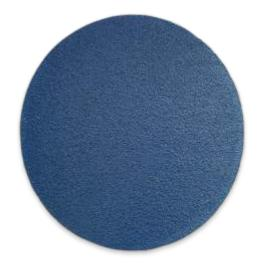
Slipmet Z velcro discs are ideal for sanding metal with hand held sanders - low alloy steel, stainless steel, high alloy steel, heat resistant steel, cast iron. Characterized by high stock removal and long life. Slipmet Z sanding discs are with Y poly-cotton cloth and velcro backing and 100% Zirconia abrasive. In standard 125 and 150 mm discs with velcro backing to attach to various sanding backing pads.
