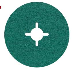
Slipfiber Z+ is made using zirconia abrasive grain with resin over resin bonding on heavy duty vulcanized fiber backing (0,80 mm), also with friction and heat resistant top size coating.
