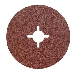
Slipfiber A- is made using aluminium oxide abrasive grain with resin over resin bonding on heavy duty vulcanized fiber backing (0,70mm).
