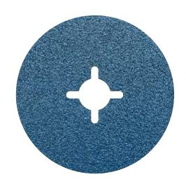
Slipfiber Z is made using zirconia abrasive grain with resin over resin bonding on heavy duty vulcanized fiber backing (0,80 mm).
