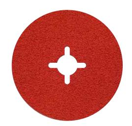
Slipfiber C is using ceramic abrasive grain with resin over resin bonding on heavy duty vulcanized fiber backing (0,85 mm), also with friction and heat resistant top size coating.
