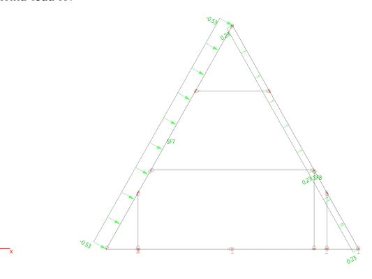
Remark: wind load on roof is calculated based on velocity pressure  $\, q_p(z) = 0,73 kN/m^2 \,$
