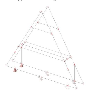
Remarks: circle is showing hinge at the end or beginning of the 1D member; on supports, square mark indicates in which direction support is
