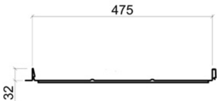
Cross section of Classic model D
