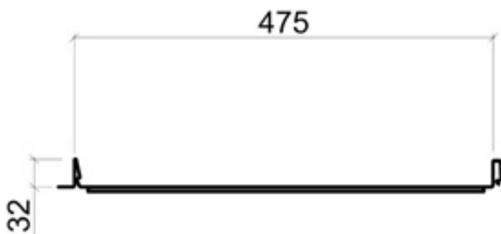
Cross section of Classic model C
