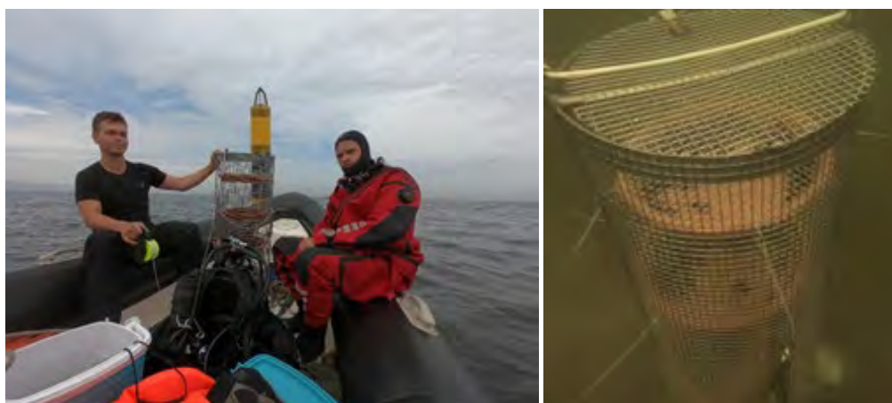
Figure 4.3.8 Installing the cage with mussels and the cage with bioindicator organisms underwater.
