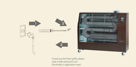
In case that you keep the heater for a long time and you want to maintain it in clean status, please power off and cool down the heater, and pull out the plug as the above picture and clean according to the following instruction.
