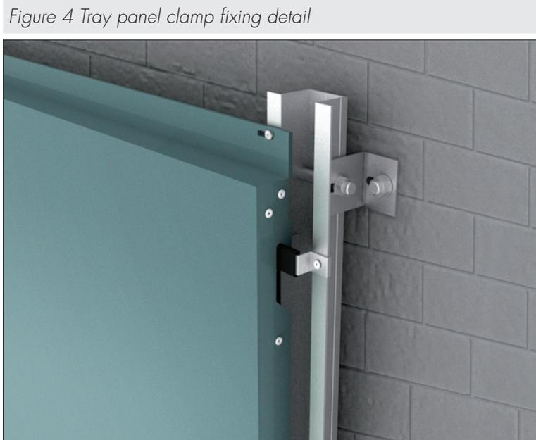
13.8 Tray panels should also be installed in ascending rows with their positions checked and adjusted as necessary as installation proceeds. The clamping pieces incorporating an EPDM sleeve are fixed to the both wings of the vertical support rail using screw fixings.
