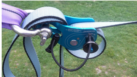
Feed bite through the shackle, make sure the webbing lies flat against the lowest webbing layer
