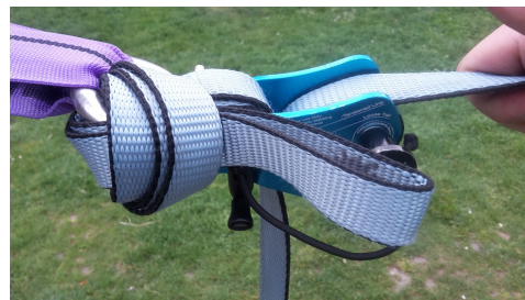
Feed bite through both wraps to finish knot
