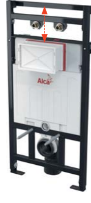
A108F/1100 Mounting frame with cistern for a waste sink with waste connection DN90/110 and faucet
