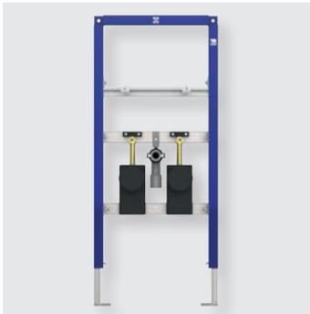
**Wash basin element INEO for single hole mixers with 2 concealed water meter units, concealed valve and T-piece for angle valve and storey distribution**
