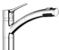
33581..75 single-lever sink mixer swivelling spout (110°) pull-out hand spray automatic diverter: shower/spray
