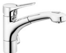
39945.62 multi single-lever sink mixer swivelling spout (110°) pull-out hand spray automatic diverter: shower/spray connection for a washing machine or a dishwasher
