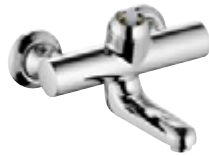
335310500 single-lever basin mixer optional for clinic or public lever ceramic cartridge with hot water limitation swivelling or lockable spout
