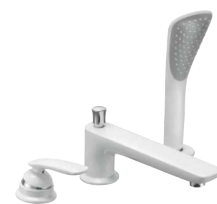
524479175 single lever bath and shower mixer DN 15 for three hole tile rim installation projection 220 mm
