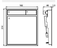
A. Base plate, B. Pair of buttons Different colour combinations possible for A and B
