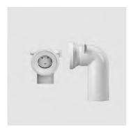
WC connecting bend 90°, DN 100, with lockable rat blocker in white PP plastic, for floor-standing WCs, with built-in mechanical rat blocker, rear side of valve clad with bite-resistant stainless steel, prevents the invasion of foreign objects to the WC, additional manual operation for cleaning by hand possible, packed in a box
