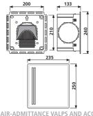
Built-in wall box with ventilair® air-admittance valve DN 70 - 100
