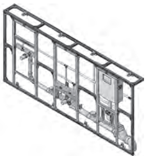
Front wall with washbasin-, urinal- and wc module with complete waste water and drinking water piping
