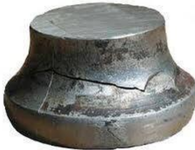
Cracked Rod Head
