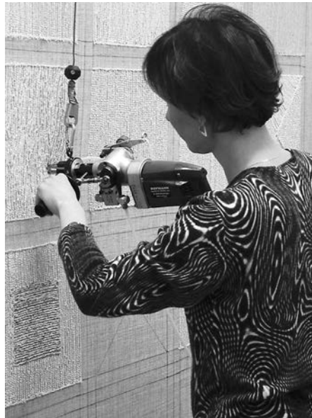
Picture nr. 1. Hand-tuft technique
