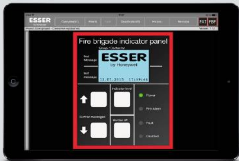
Standardized user interface in the form of a fire department display panel
