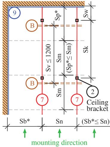
b) Configuration of profiles for alternate mounting of module 600x600mm
