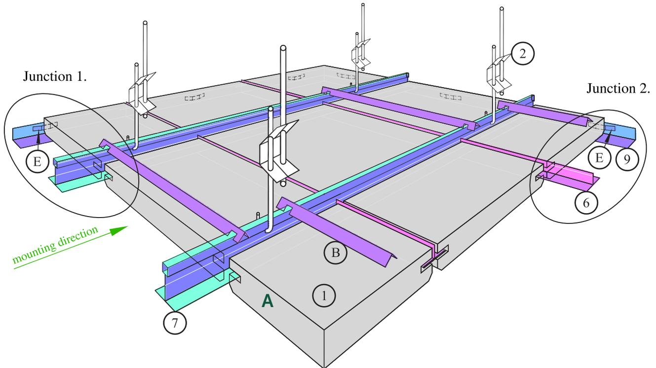
T-profile suspended ceiling frame is manufactured by a number of manufacturers. CEWOOD panel mounting instructions have been elaborated specifically for the frame element system DONN DX-T35. Bearing profiles T 35/38.
