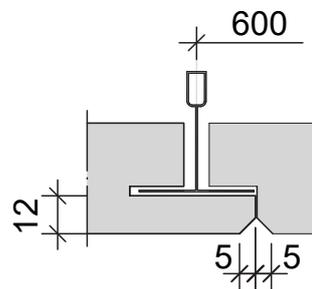
CEWOOD panels with edge profile P5S are mounted on T-profile frame. The structure is dismountable.
