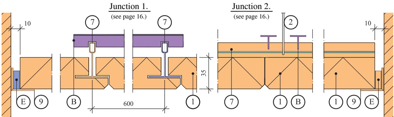
**Fig. 7.5. Orientation of quick suspension mounting.**
