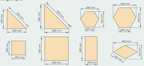
Design tiles are installed by gluing. Detailed instructions can be found in the "Downloads" section under the file "Glue selection instructions and surface preparation". For more massive panels, for example in the size of 580x580 mm, especially when mounted on ceilings, additional screw fixing is recommended. In this case, refer to the file "Screw installation guidelines for panels".
