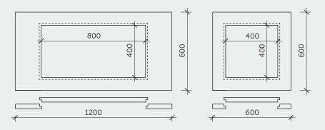
(!) Inspection hatches can be integrated into both CEWOOD panels and Barcode panels and fixed with screws to a metal or wooden substructure, or into a T-profile grid. Panels with inspection hatches must be installed in accordance with the CEWOOD panel installation requirements.
