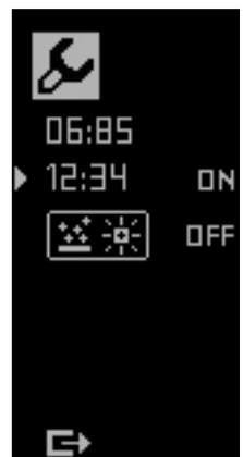
The icon shown on the timer row is either on or off (depending on whether the timer is switched on or off). In blinking mode the on/off icon can be changed by using buttons X/Y. Press OK button to switch the timer on, if there is icon "ON" behind the time reading. You can select on/off icon by pressing button P.
