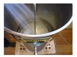
Add 12 L/23 L/55 L brewing water – for 20 L to approx. 2 cm below the upper marking on the tie rod or filling level indicator.
