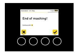
After completion of the programmed brewing phases, another signal tone is emitted. This will also be acknowledged by pressing the *Select* button. The pump switches off and you are prompted to start purifying Remove malt pipe. Purification means separating the crushed malt from the beer wort. Purifying with the Braumeister is a relatively easy, fast and clean exercise, compared to many other home brewing methods, and represents a central concept of the Braumeister. Remove
