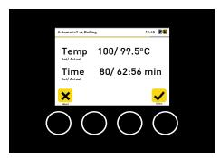
As described in the previous section, automatic brewing continues and the hops boiling process is started. The display again shows the time and temperature of the phase. As the target temperature of 100°C cannot always be reached, timing starts after a waiting period of 3 minutes without increase in temperature. When pressing the *Select* button during the automatic mode, the target temperature and target time can be corrected or changed. Wort is boiled during this phase. On the one hand,
