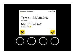
Once you have filled the malt, acknowledge it by pressing the *Select* button. For safety reasons, you will receive the prompt "Malt filled in?" And by pressing *Select* the actual brew process commences with the Braumeister. The pump and the heating switch on. The wort rises up in the pipe and overflows. The cycle has begun and the malt is washed out by means of transfer pumping in the next phases.
