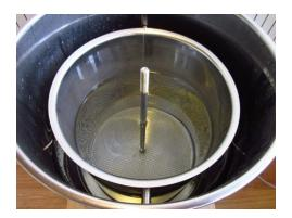
When the mashing-in temperature has been reached, a signal tone is emitted; press *Select* to acknowledge it. Then insert the malt pipe (with pulled-on seal facing downwards). Ensure that the seal is centred on the malt pipe and sits absolutely flush on the vessel base. Slide in the filter plate to the lower edge (pipe facing up). Then insert the fine sieve (position at bottom of water).
