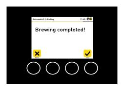
Once the boiling time has elapsed, another signal tone is emitted, indicating the end of the brewing procedure. Use the *Select* button to acknowledge it. The heating switches off.
