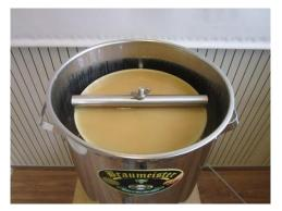
Press the *Select* button to continuethe Automatic mode. Lightly coloured brewing water rises up and spills over. The cycle has begun. The next brewing phases take place fully automatically, as programmed. During some of the brewing phases, the control causes a short pump break to reposition the malt. The display shows the actual and the target temperatures as well as the target and actual run time for each phase.
