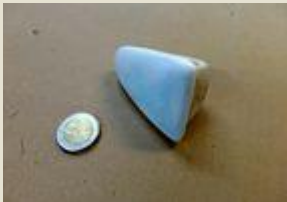
polishing stone (ceramic or natural stone, minimum hardness 6 on the Mohs scale)
