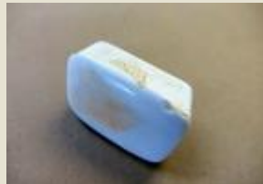
polishing stone (ceramic or natural stone, minimum hardness 6 on the Mohs scale)
