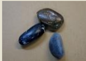
polishing stone (ceramic or natural stone, minimum hardness 6 on the Mohs scale)
