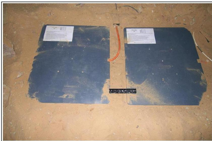
**Photo 1.** Installation of visitor counting equipment (counter mat) into Piusa cave. Counters were covered with sand, so they are not detected by visitors. Similar counters were installed into other sites as well. *Photo by Lauri Lutsar.*
