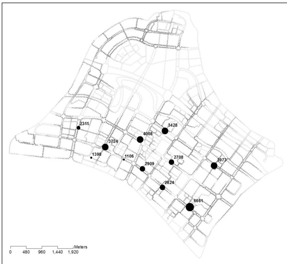
Figure 7. Estimated patronage of existing clusters with demand originating from MRT walk routes. Total patronage in town = 35,055 households. Beta = 0.001; search radius = 3000 meters; alpha = 0.37.
