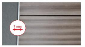
Between the outer deck and immovable object (wall, house, etc.). Leave the space: - <u>15 mm</u> if the board clings to the object in longitudinal direction and <u>7 mm</u> if the board is adhering to the object width direction.
