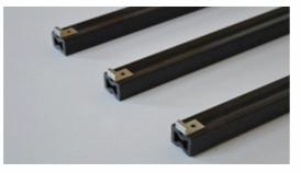
Start with placing support beams on firm ground of your choice. The support beams have to be placed with <u>35 - 40 cm</u> space between them. In case you are going to place some heavy weights on your terrace the space between support beams has to be <u>30 cm</u>. Otherwise the max allowed distance is <u>40 cm</u>!
