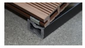
Attach the outer decking board with metal fastener, tightening it to the support beam with stainless steal screw. Before bolting it is necessary to place metal fastener at the midpoint of support beam.
