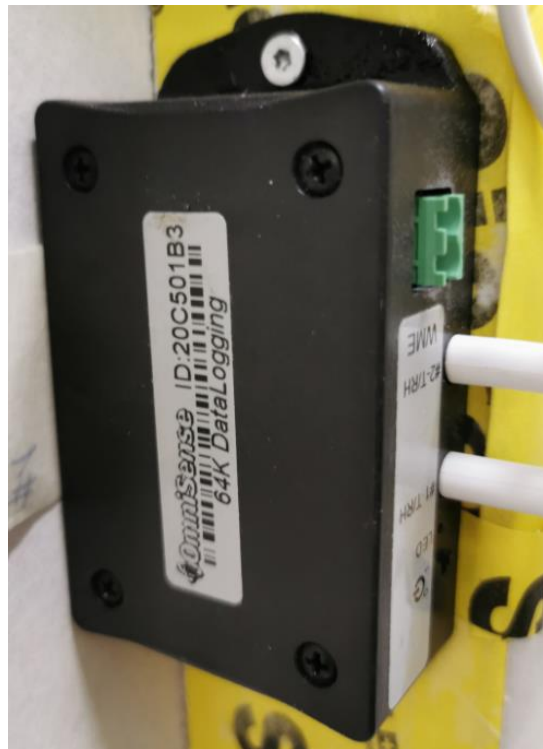
Figure 2.2 Transmitter used in Omnisense system
