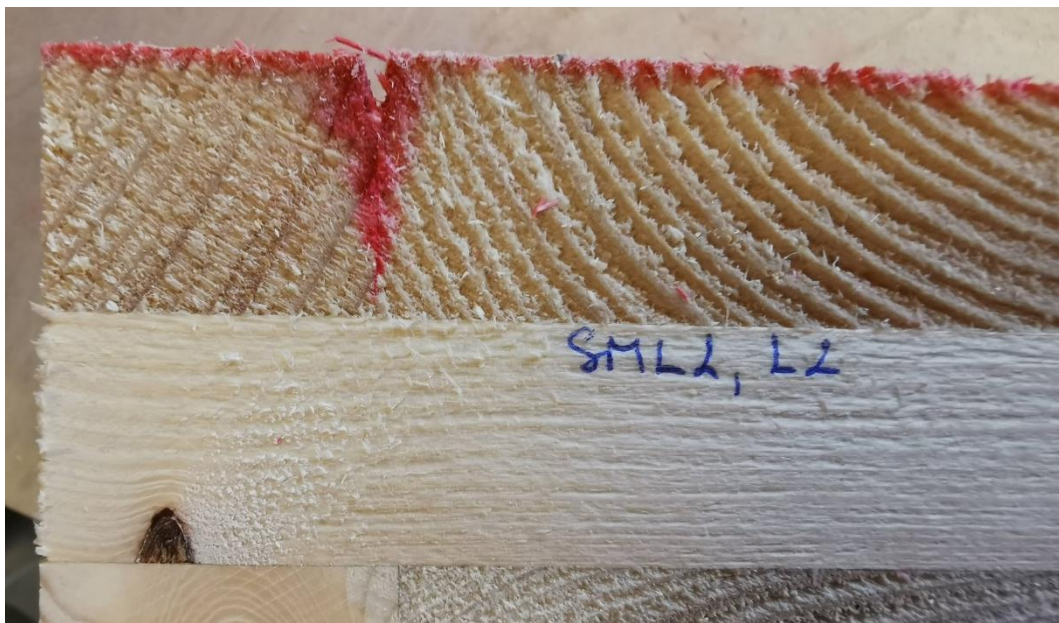
Figure 3.11 Sample with mastics and tape covered edges and incisions. Here is shown the incision and how much water has absorbed through it.
