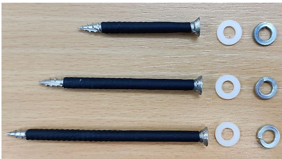
Figure 2.4 Insulated screw electrodes with plastic and spring washers
