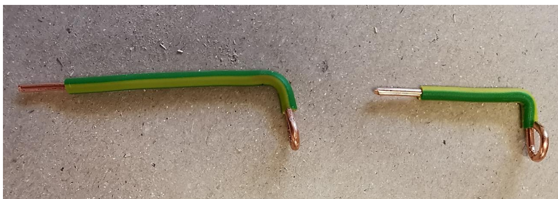
Figure 2.3 Insulated copper wire electrodes
