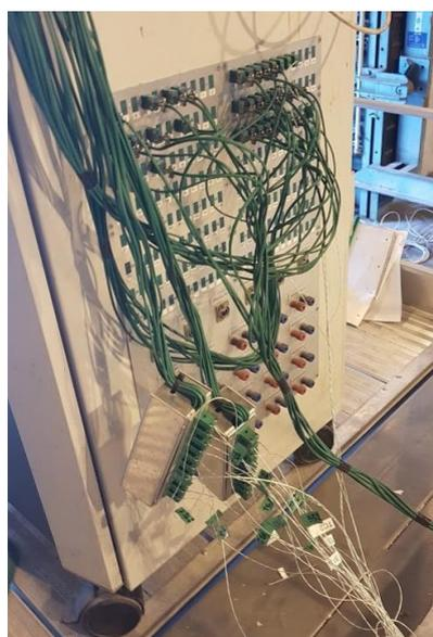
*Figure 4.1-14 Thermocouple connectors*
