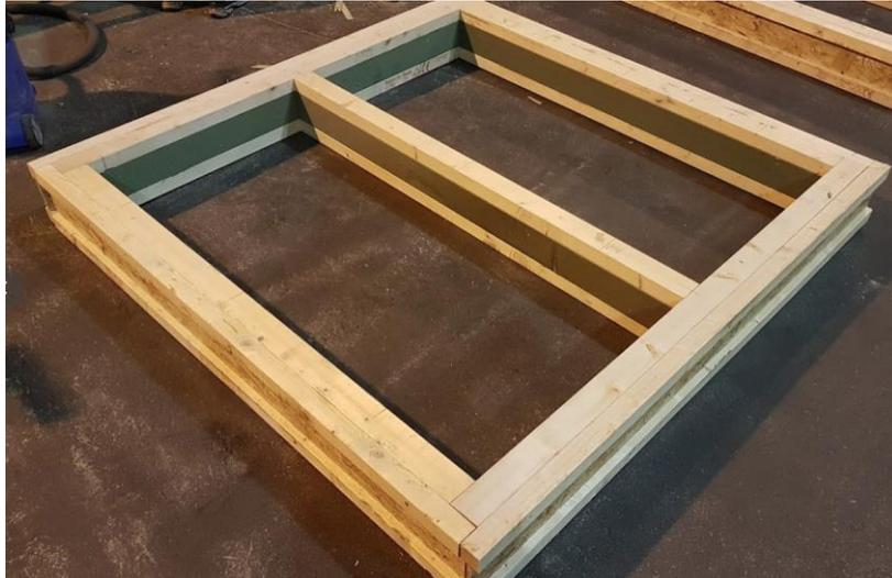
*Figure 4.1-3 Framework of the specimen*
