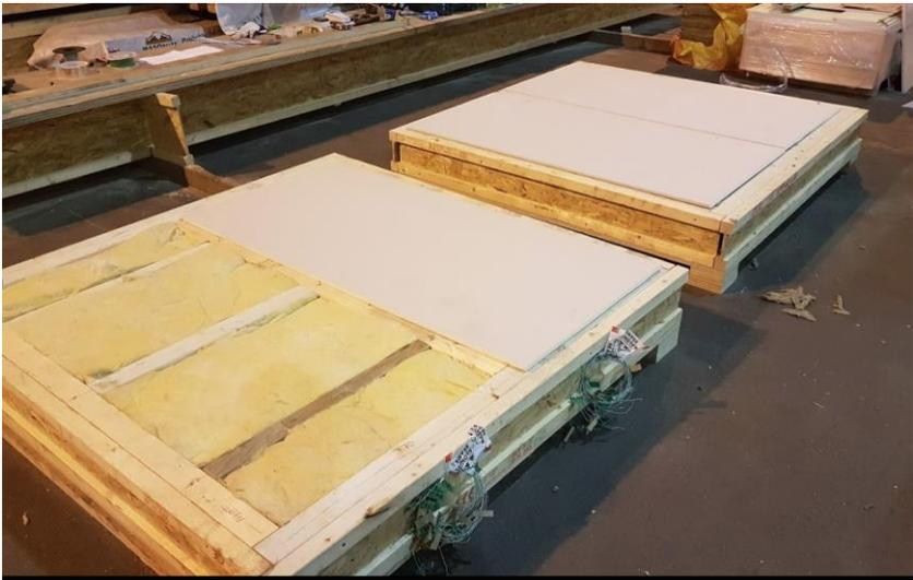
Figure 4.1-8 Construction of the specimen-installing the plasterboard
