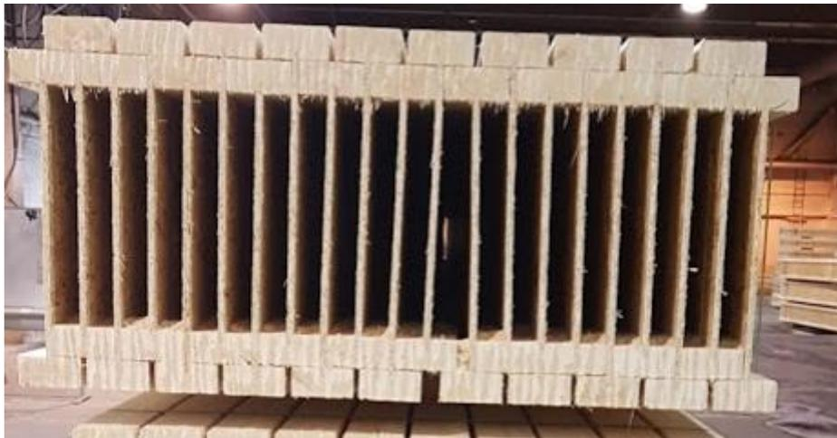
Figure 3.1-2 I-joists stacking
