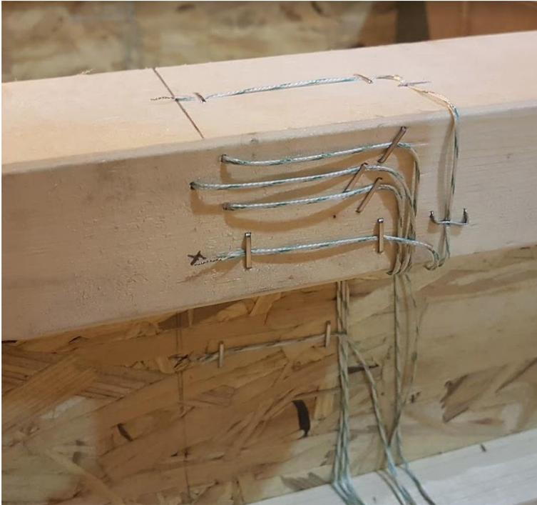
Figure 4.1-12 Location of the thermocouples – side view
