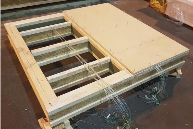
Figure 4.1-6 Construction of the specimen – thermocouples installed, screwing in the wooden particle board
