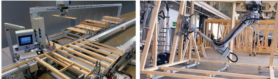
*Figure 8. Left: production of a stud frame at a framing station (Kaufmann et al., 2018); right: robotically controlled room module assembly (Huß et al., 2018)*
