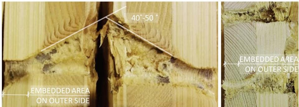
Figure 63. Left: embedded area of long SBD; right: the same for long WS
