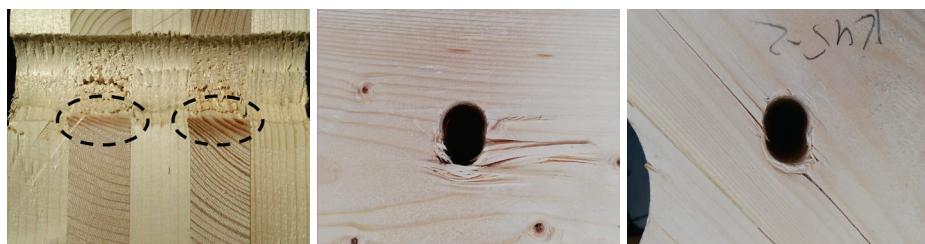
Figure 51. Left and middle: densification in crossed layers; right: embedment by sample loaded at an angle of 45 degree
