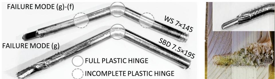
Figure 64. Left: dowel failures in connection; right: embedded area under the drill tip SBD
