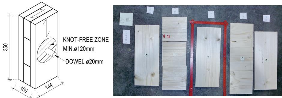
*Figure 30. Left: measurements of specimens and knot-free zone; right: visual selection of layers for 5-layer cross-laminated timber specimen*
