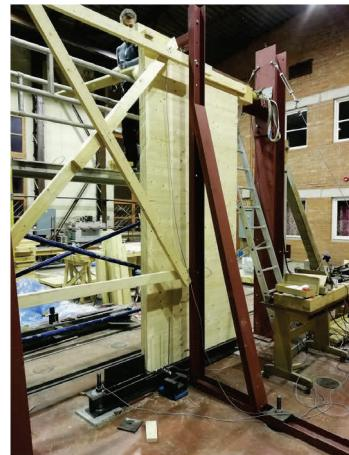
Figure 37. Line-connected cantilever shear wall
