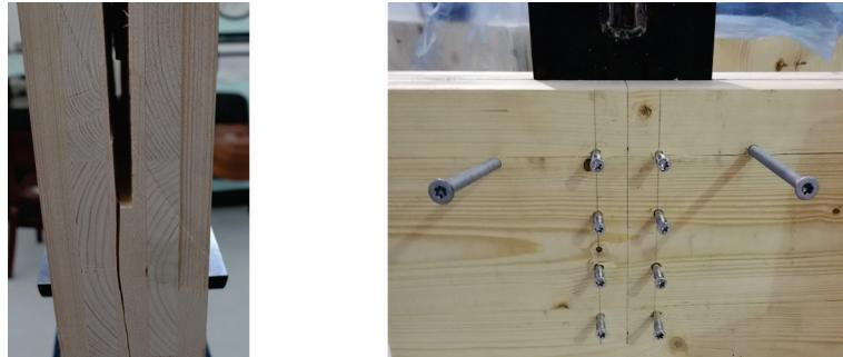
Figure 62. Left: splitting of the whole connection; right: reinforcement to avoid splitting
