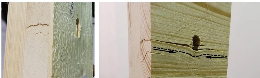
Figure 54. Shear failure in crossed layer due to the rope effect
