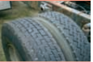
All tyres installed on one axes must have the same thread pattern and the tyres and rims shall meet the sizes specified in the technical specification.
