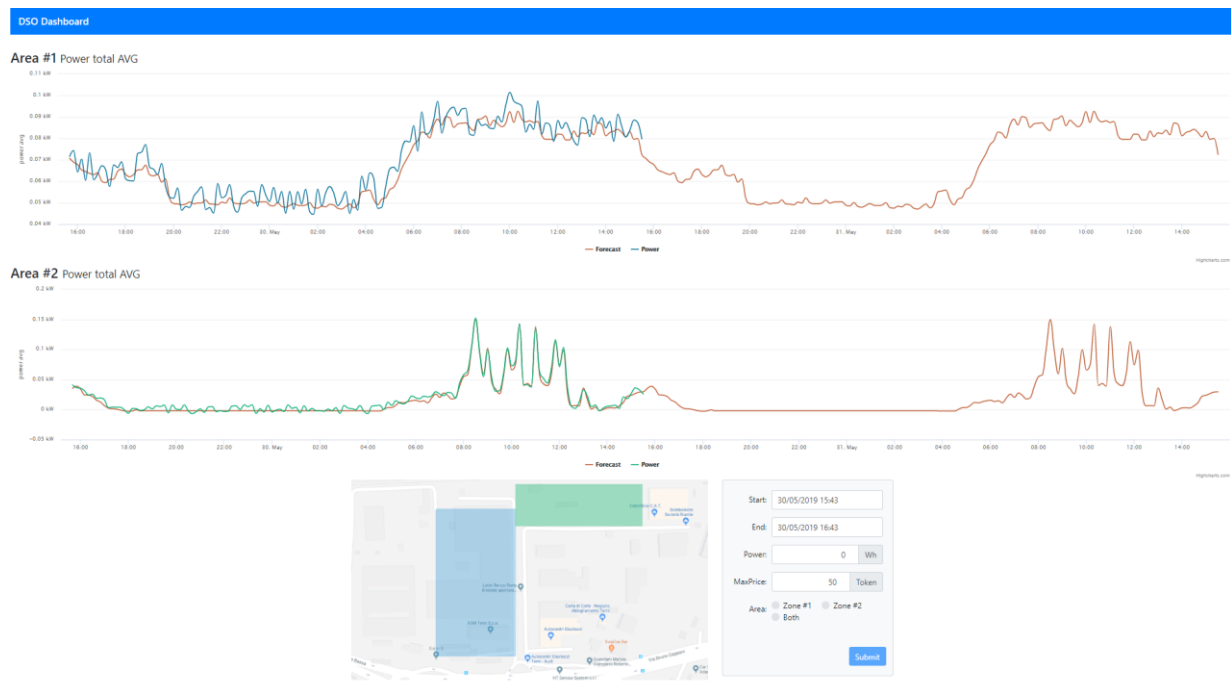
Figure 37. DSO dashboard showing forecast, smart meters data and the request creation form.
