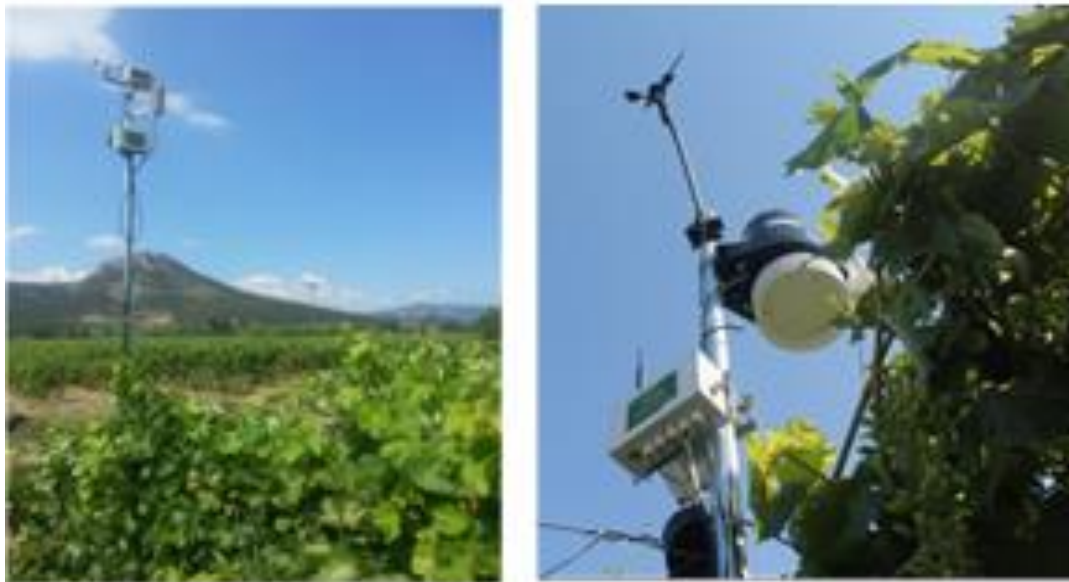
Figure 10. SynField HN and sensors deployed in a vineyard field in Soulinari (Kiato region)
